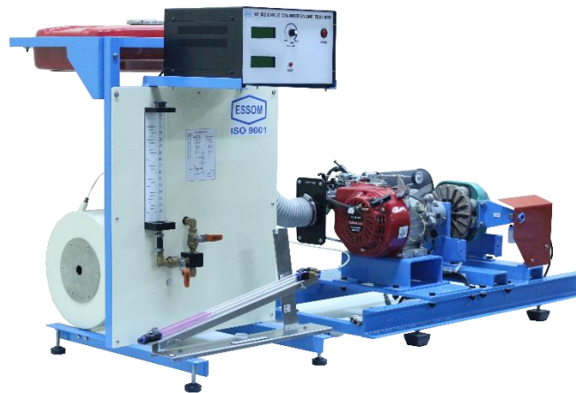
MT 502E with gasoline engine and eddy current absorber
