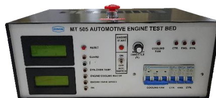
Instrument box for water absorber
