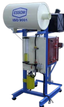
Airbox, fuel tank Thermostatic tank and fuel flow measuring device
